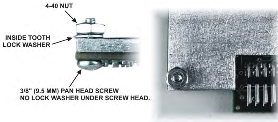
Figure 25. Stiffener Plate Fastener on KSYN3 Board.
