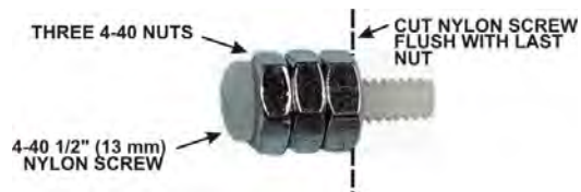
Figure 13. Cutting 1/2" (13mm) Nylon Screws.
